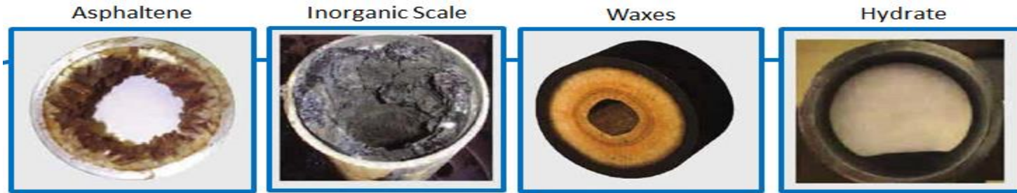
Types of oil pipe obstructions.
